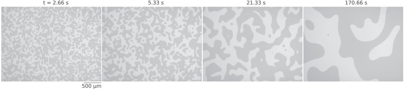
FIG. 2. Configurations of the ordering of TNLC during a relaxation toward the equilibrium. The dynamics was triggered by a virtually instantaneous electrical switch (at  $t = 0$  s) from a spatiotemporally chaotic called DSM2 toward the two-phase competing, equilibrium state. Different shades of gray correspond to twists of opposite handedness in the nematic director field. See also supplemental videos 1 and 2 [121].
