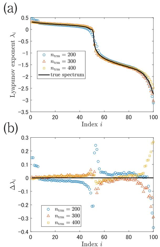
FIG. 4. The spectrum of the Lyapunov exponents  $\lambda_i$  for the globally coupled limit-cycle oscillators. (a) The spectrum evaluated by the proposed method (symbols) for different choices of the trimming threshold  $n_{\text{trm}}$ . The black line indicates the true spectrum  $\lambda_i^{\text{true}}$  obtained by the standard QR decomposition method. (b) The estimation error  $\Delta \lambda_i := \lambda_i - \lambda_i^{\text{true}}$ .
