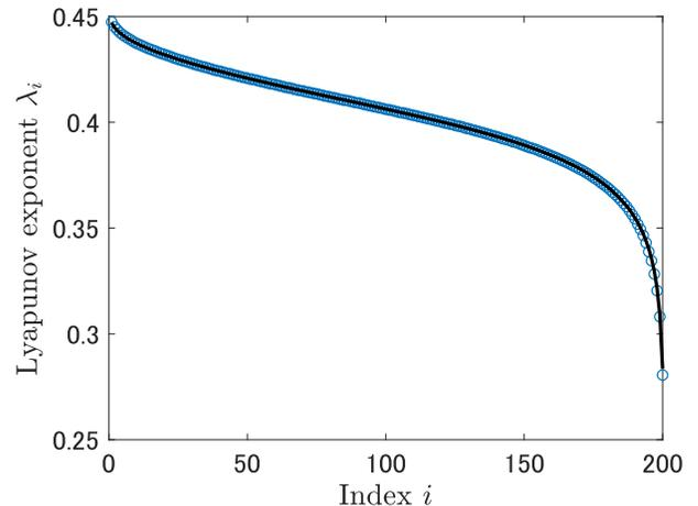
FIG. 2. The spectrum of the Lyapunov exponents  $\lambda_i$  for the globally coupled logistic maps, evaluated by the proposed method (blue circles). The black line indicates the true spectrum obtained by the standard QR decomposition method.
